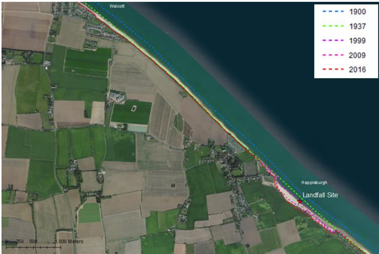
Figure 2-4: Cliff erosion between Happisburgh and Cart Gap
